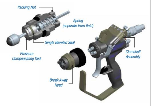
The Graco RS Gun also has a break-away front head, which allows for quick and easy maintenance. Phasing (lead/lag) has been addressed in the design and is factory set. No longer does the end user no longer have to make adjustments to the gun when the needle packing is tightened or the needle assembly replaced. The needle assemblies are also protected from overspray by a clamshell assembly.
